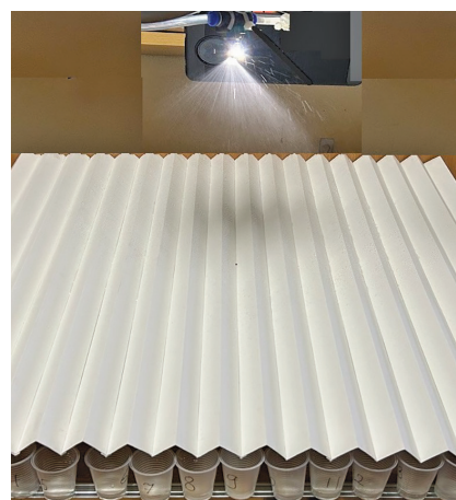
Figure 6. Determination of the spraying spectrum for one nozzle Source: compiled by the authors
